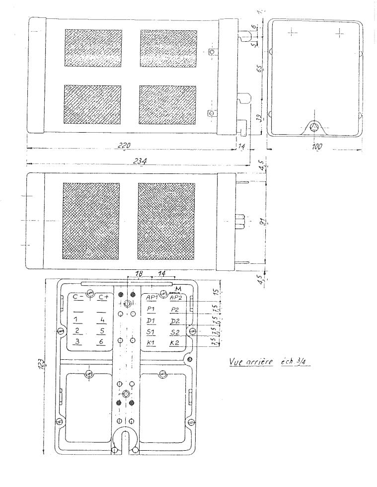
IB179 Page 17 Fig. 3.6.2. Outline Drawing of Transmitter type NCO EGT 600
