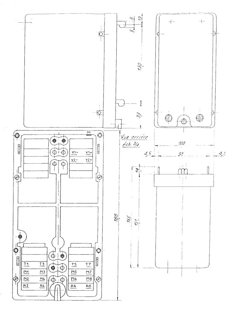
IB179 Page 23 Fig. 3.6.8. Outline Drawing of Track Relay type NCO CVTH 2.4.0.4.
