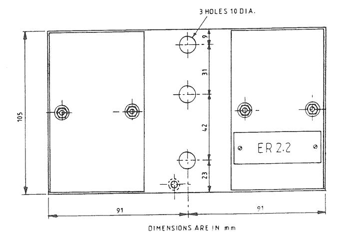
IB179 Page 20 Fig. 3.6.5. Outline Drawing of Resistance Unit type ER 2.2
