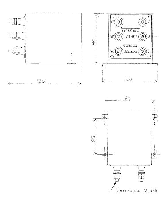
IB179 Page 19 Fig. 3.6.4. Outline Drawing of Track Transformer type TVTHD2
