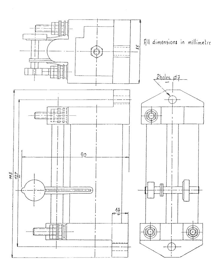
IB179 Page 21 Fig. 3.6.6. Outline Drawing of Variable Resistance type RK 40
