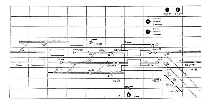
Mosaic diagram, showing part of a control panel and including an interlocking that is remotely controlled.
