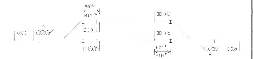
If Signals B, C, D & E are positioned 50 yards from the "fouling points" of connections it is possible to allow two trains to enter adjacent lines of the Passing Loop at the same time using "delayed yellow" aspects.
