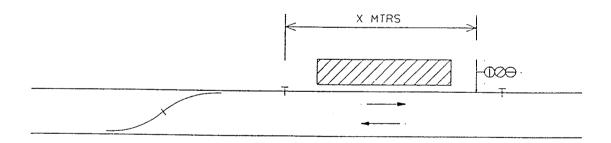
(b) Standing room should ideally be 16 feet (4.88 metres) from the Fouling Point but this measurement may be reduced if a detailed calculation is carried out (see SSP No.36 for details).
