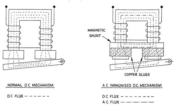
To overcome the problem in DC traction areas AC track circuits are used. There are two principal methods of immunising AC track circuits from the effects of stray currents from electric traction systems:-
