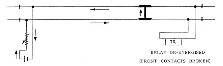
Current flows from the battery through the variable feed resistance to the positive track rail.
