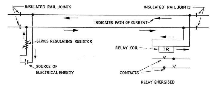
Current flows from the battery through the variable feed resistance which regulates the flow of current via the positive track rail to the track relay. It passes through the relay winding, causing the relay to be energised and to close its front contacts, from where it returns through the negative track rail to the battery.
