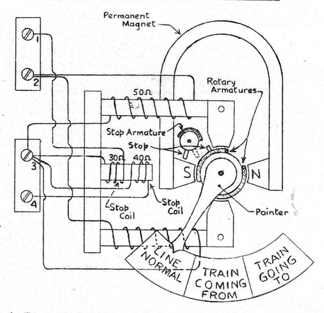
1. The two 50  $\Omega$  Operating Coils are connected in parallel between terminals 2 and 3, thus giving a joint resistance of 25  $\Omega$ .
