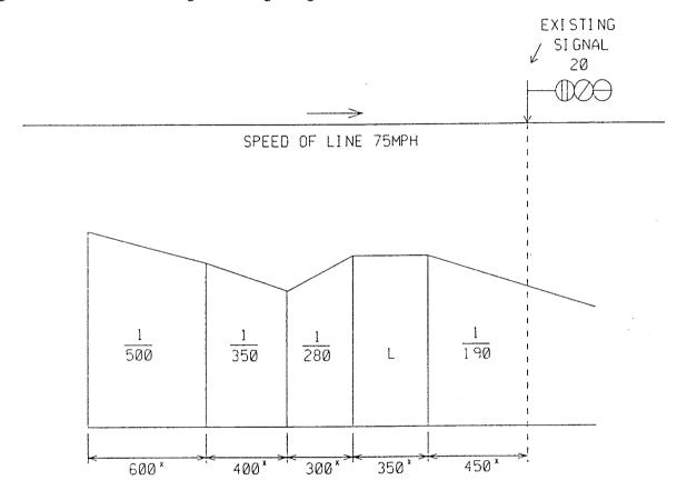
When the new signal in rear of 20 is showing a yellow aspect this signal must be placed at SBD plus the parameters previously quoted (between 1.1 & 1.5xSBD) must be taken into account.
