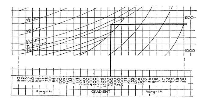
Theoretically Signal 1 could be placed closer to Signal 2 but in practice it has been suggested to aim to place the Distant Signal between 1.1xSBD and 1.5xSBD. This flexibility of measurement can have benefits when taking site considerations into account. ie. accommodating existing signals, actually siting the signal because of Signal Sighting Committee recommendations and signal adjustment to a preferred "Headway" pattern.
