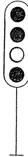
CAUTION Be prepared to stop at next signal which is now at RED .
