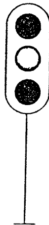
CAUTION Be prepared to STOP at next signal which is now at RED .
