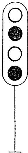
PRELIMINARY CAUTION Prepare to pass next signal at restricted speed & to find it showing one YELLOW light
